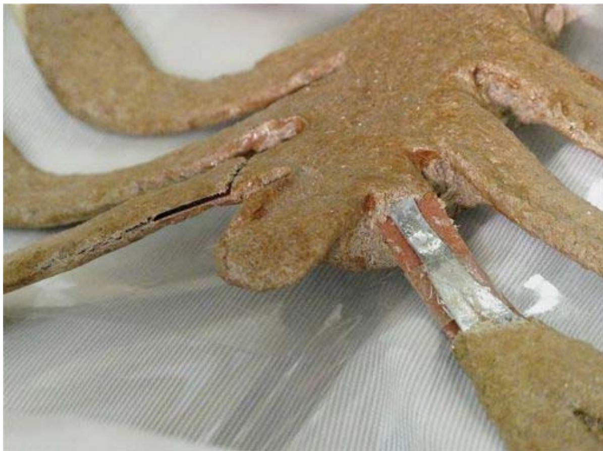
Figure 14: Original steel insert had been covered with epoxy, which cracked and broke during the fall.
